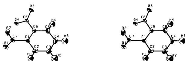
Fig. 1. Stereoscopic view of the phthalate group. The thermal ellipsoids are the 50% probability surfaces.
